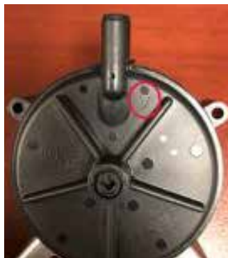
Pressure switch side "V"
