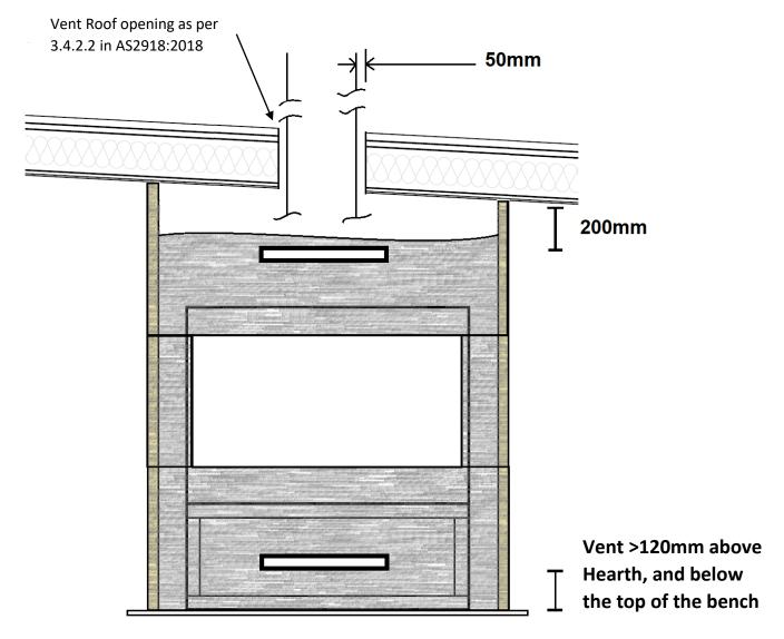
Vents included below Zero Clearance box and below Inbuilt cavity cap
