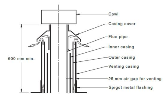
Options 2: Chimney Chase construction and side vent.
