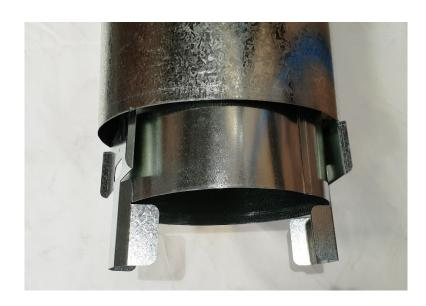
The 10" slides through the top of the Zero Clearance Box and sits above the heater resting on the brackets. The 10" MUST be sealed with a flexible sealant around the top of the Zero Clearance box to stop heater air coming into the chimney chase cavity.
