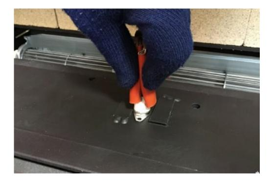
Rotate the Thermostat under the tabs to lock in position.
