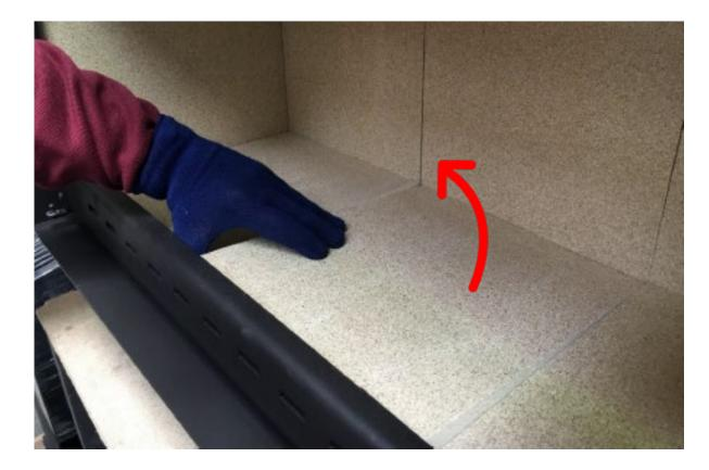
2. Remove the vermiculite base bricks from the floor of the firebox.
