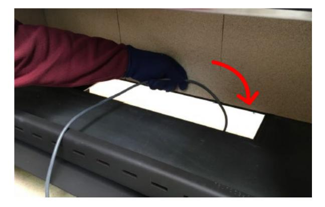
Pass the toggle switch cables through to the front.
