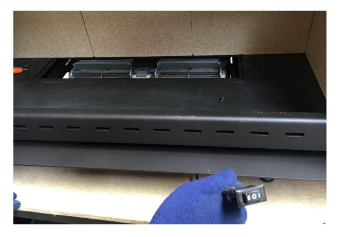
Pull the switch forward toward the front, ready for mounting position.
