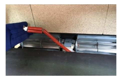
Fix the fan in position with 2 screws on each end.
