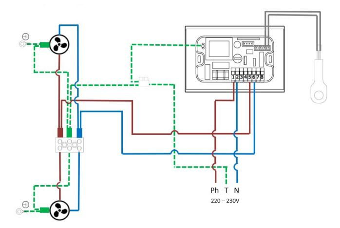
1 And 5 Wires – BLUE 2 And 6 Wires – BROWN Dotted E wires = Earth
