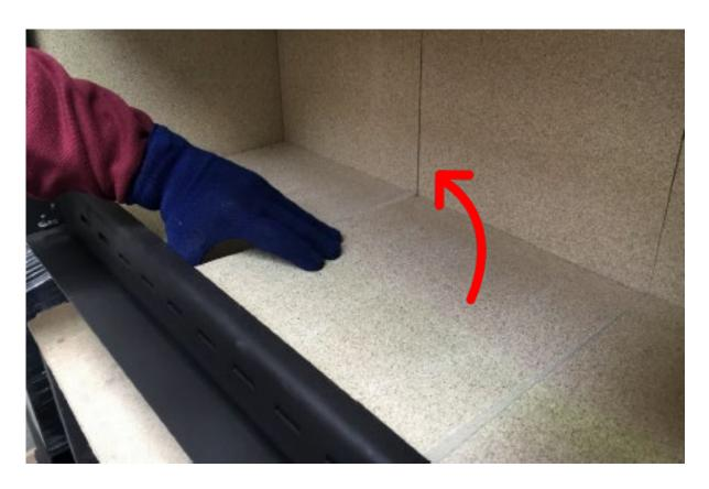
Undo the screws and remove the fan access cover (flat steel plate). Single sided shown. Double sided has each fan running front to back on LHS and RHS.
