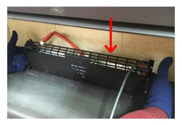
Ensure there is NO Gap in the Top between the fan and the heater.
