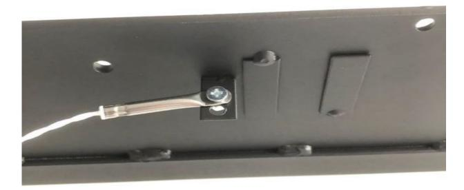
For appliances built before February 2020, use the supplied adaptor bracket, to fix below the Thermostat tabs on the underside of the firebox, and fit the thermocouple wire to the adaptor bracket.
