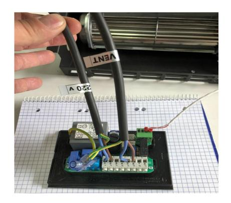
1 And 5 Wires – BLUE 2 And 6 Wires – BROWN Wires through Blue Joiner, Earth = Yellow and Green stripe
