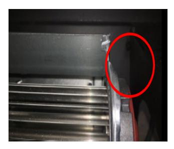
Fix the fan in position with 2 screws on each end.
